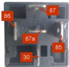
Bottom of Relay Wiring Diagram
